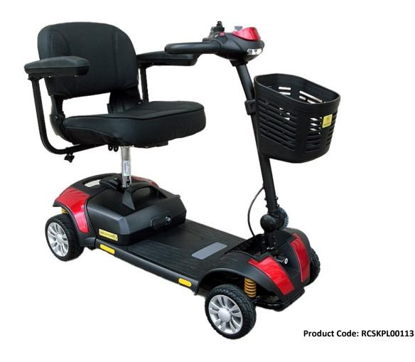
This compact scooter is great for confined spaces, both indoor and out. It comfortably fits in the back of a small hatchback. The tiller folds down and the seat lifts off.
