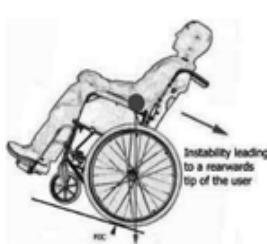
Figure 6 Unstable (slope too steep)
